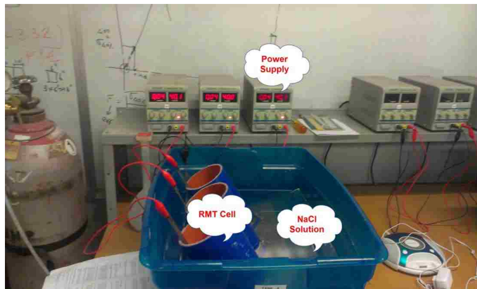
Figure 3.14: Rapid Migration Test Setup
