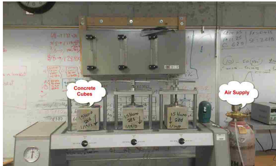
Figure 3.11: Concrete Water Penetration Testing Apparatus
